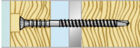
Installation in sheet metal/steel studs (max. 2.0 mm), with wooden stud reinforcement, directly without pre-drilling
