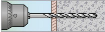
1. Drill the hole. Hole diameter is equal to the nail diameter.
