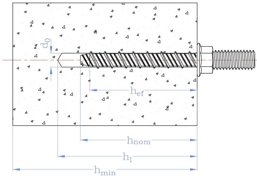
**Drawing A3.** Installed condition for anchors EUS - SSD, EUS - SSI, EUS - SSF, EUS - SSO, EUS - SSU, EUS - SSG, EUS - SSQ, EUS - SSV and EUS - SSG2
