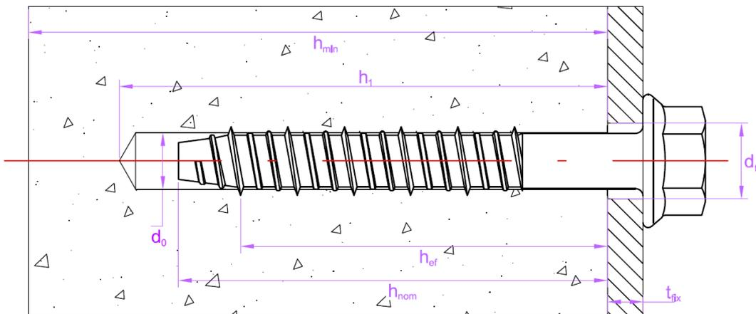
**Drawing A1.** Installed condition for anchors EUS - SSW, EUS - SSR, EUS - SSP, EUS - SSK, EUS - SSH, EUS - SSX, EUS - SST, EUS - SSN and EUS - SSC.
