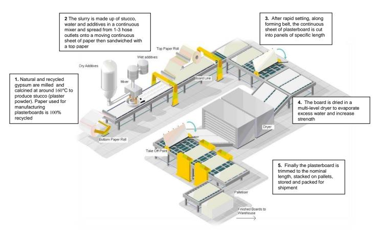
Figure 2: Manufacturing process flow diagram. The manufacturing process is described in detail within the diagram.
