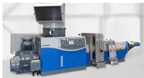
Figure 3. Machine to make new granulates of the spillage.
