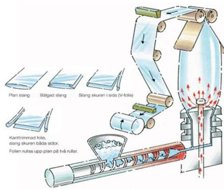
Figure 2. Sketch of the manufacturing process.
