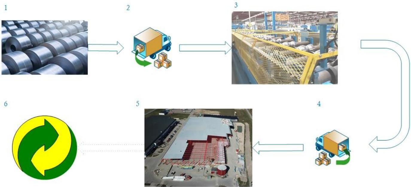
The steel coils (1) are produced at the steel manufacturer and transported to Lindab Profil Förlöv by truck (2). The high profile is produced in a roll forming machine (3). The production is a pull system (produced to customer order) to reduce waste in all parts of the life cycle. Transport to customers are done by truck (4) to the building site where the customer assemble the product (5). The usage phase is excluded in this EPD, it is why the next step is demolition and recycling (6).
