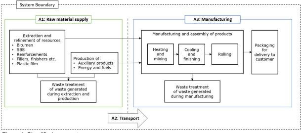
Figure 1. Simplified process tree.
